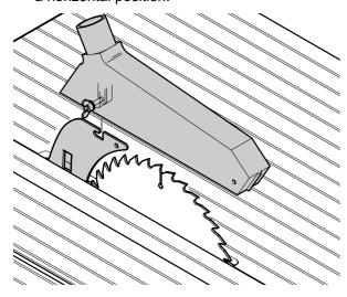
If you are using a dust collector, connect the blade guard's dust spout with the dust collector as well.
